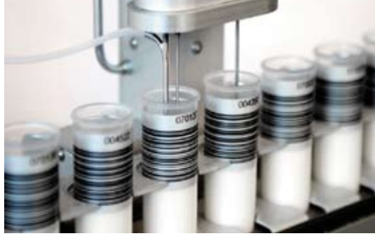
FTIR analysis determining the amount of fat, lactose, and solids content.
